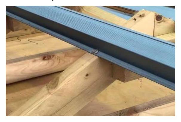
**BattenMan's 40mm Roof Battens** (Roof purlins) are a direct replacement for timber purlins. These 40mm battens are specifically designed for use with Longrun Roofing profiles and wall claddings in conjunction with wood and steel framing. With spans of 1200mm at 900mm spacing's they can be used in extra high wind zones and where snow loads are present. Being made from 0.75mm. G550 Z275 high tensile steel means it won't rot, burn, splinter, warp or twist!
